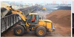
LW800K loader is loading lead zinc ore powde and coal powder in Wenzhou port
